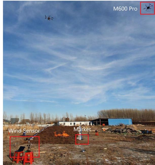
Figure 1: Burning experiment configuration. Shown from left to right are a set of wind sensor (only one of all sensors is framed), a marker point (only one of all markers is framed) and the M600Pro UAV with the infrared camera.
