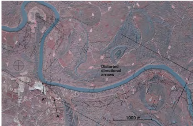
Figure 6: Initial georeferenced map near GCP 10 in Figure 3 showing problem of impossible river position well to south of high bluff. Note complete directional arrows on left but distorted one on right where the two sheets were edge matched by using the river banks as most critical junction. Point A on map indicated a small valley on the bluff which is located somewhere near point A' on the photograph. The base layer shown is the 1999 aerial photographs (SCDNR, 2014a).
